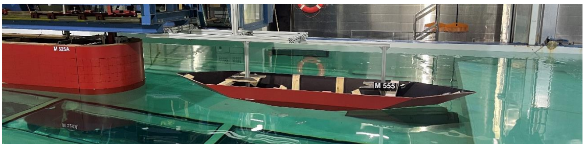
Figure 2-1: Test arrangement, icebreaker.
