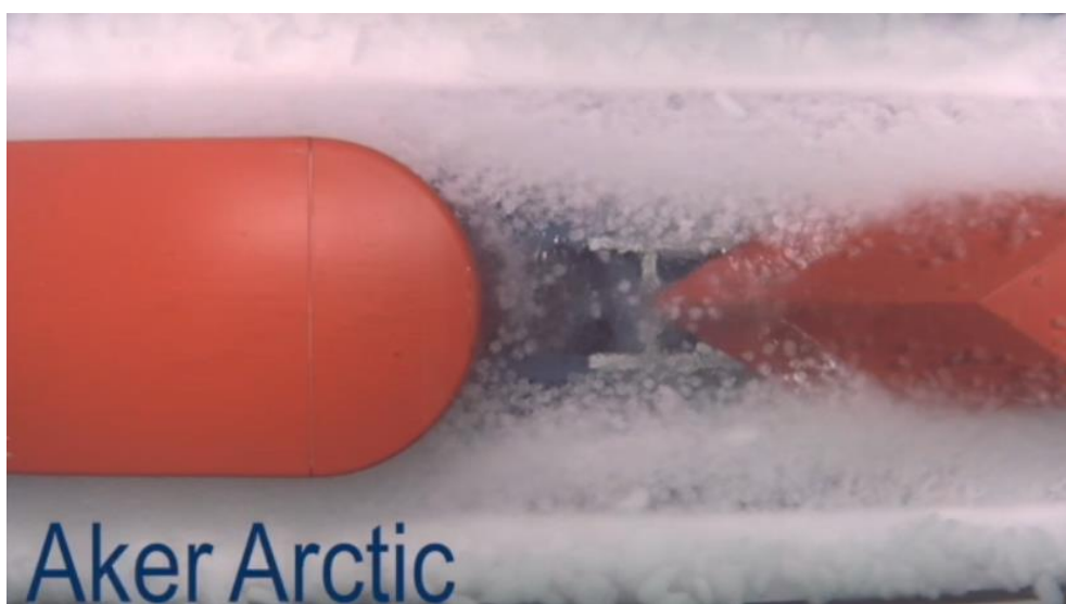
Figure 3-6: Ice accumulation between the models at 8 kn, 24.0 m icebreaker.
