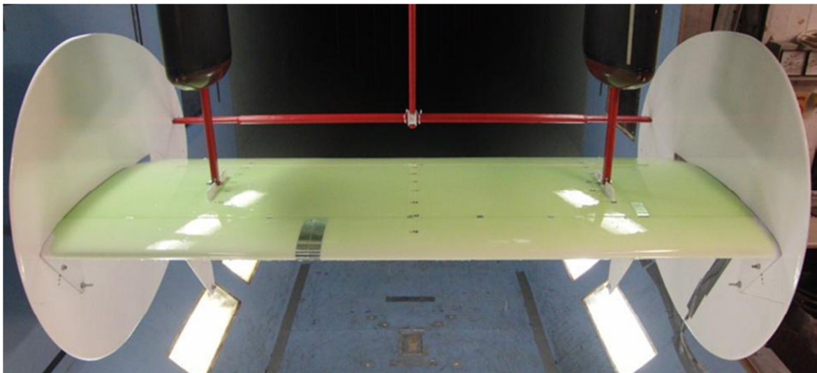
Figure 1. Rotating wing section model in wind tunnel.
