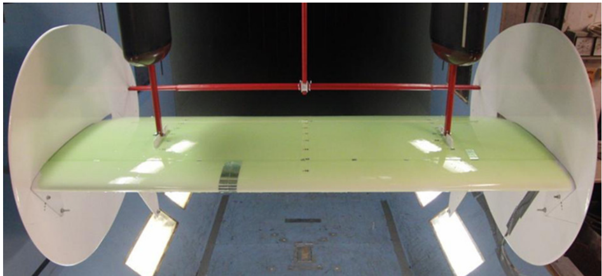
Figure 1. Rotating wing section model in wind tunnel.
