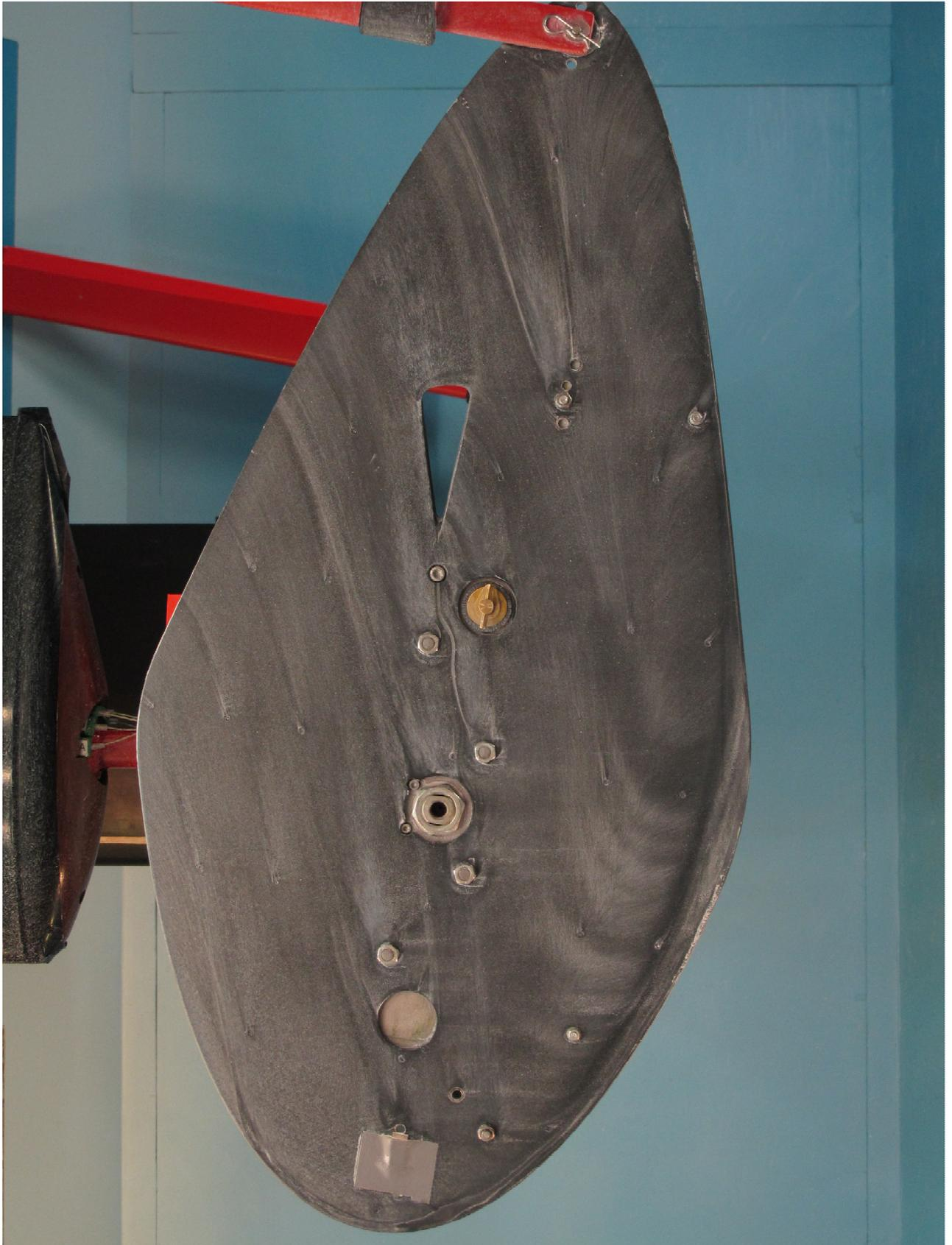
**Figure 33.** Oil flow pattern on the end plate of the HL-CRM Mod wing model at  $Re=1,3$  million.
