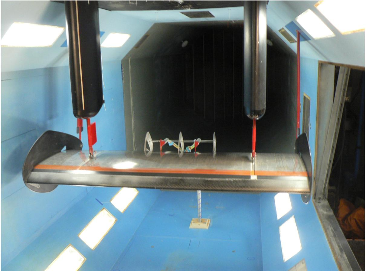
**Figure 23.** Overview of the wing model covered with PVC plastic sheet.
