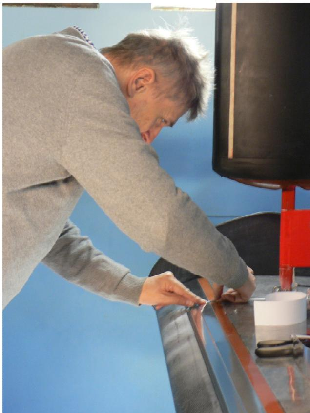
**Figure 24.** Installation of aluminum tape over the PVC plastic sheet fore edge.
