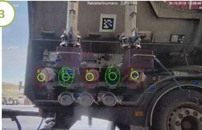
Server algorithms for detecting vehicles and tracking loading arm connections to compartment vents.
