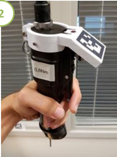
In-house designed & 3D-printed marker and LED add-on.
