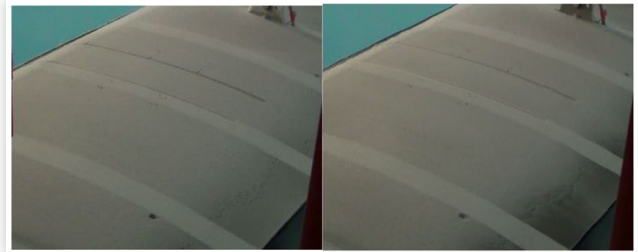
FIGURE 17 Video snapshot from the upper side of HL-CRM Mod wing section model just after rotation (left) and 60 s after rotation (right). Test section air temperature is -0.6\text{ }^{\circ}\text{C} and initial frost thickness k/c = 3.27 \cdot 10^{-3} . There is slight darkening observable at the trailing edge area.
