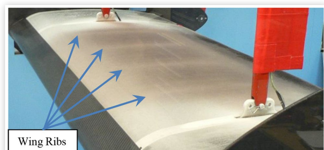
FIGURE 14 Frost on HL-CRM-Mod wing section model.
