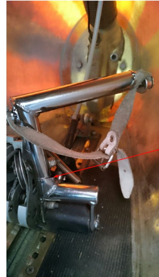
OH-733 Grob G103 Acro front pedal fracture (right) and fatigue crack (left)
