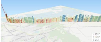
Figure: Galileo signal strength nearby Nahkialanvuori hill, Toijala (dB).
