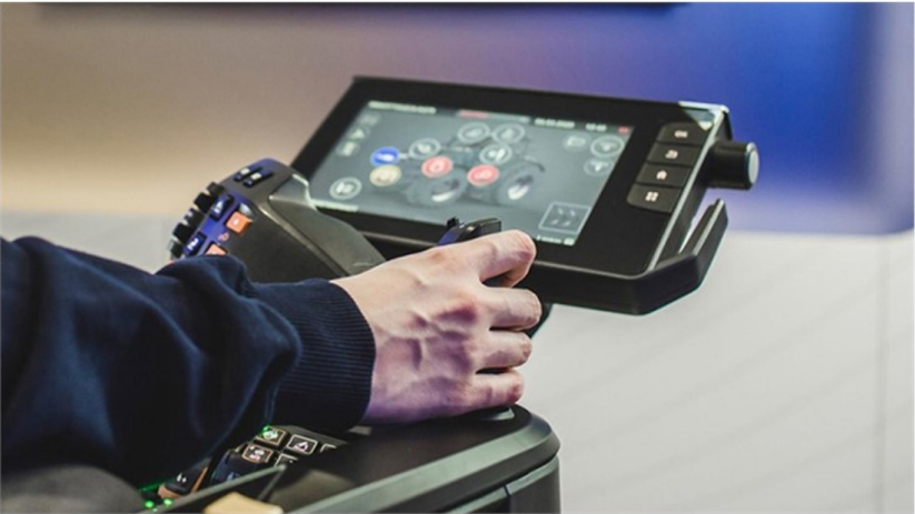
Valtra and Elisa have been working on a remote-controlled tractor that allows one to operate the machine from as far as 100 kilometres away via 5G network signals. (Photo courtesy of Valtra)
