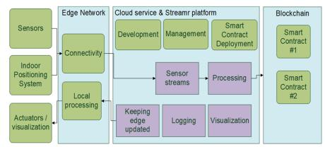
Demonstration based on orientation sensors, UWB positioning, Streamr platform for building backend applications and Ethereum blockchain
