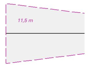
*Line of the track, fairway area and the safe clearance depth of the fairway area, shown as the international symbol of minimum depth on a printed chart.*
