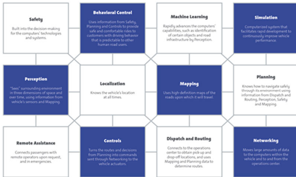
Figure 13. The building blocks of the automated driving system (General Motors 2018)
