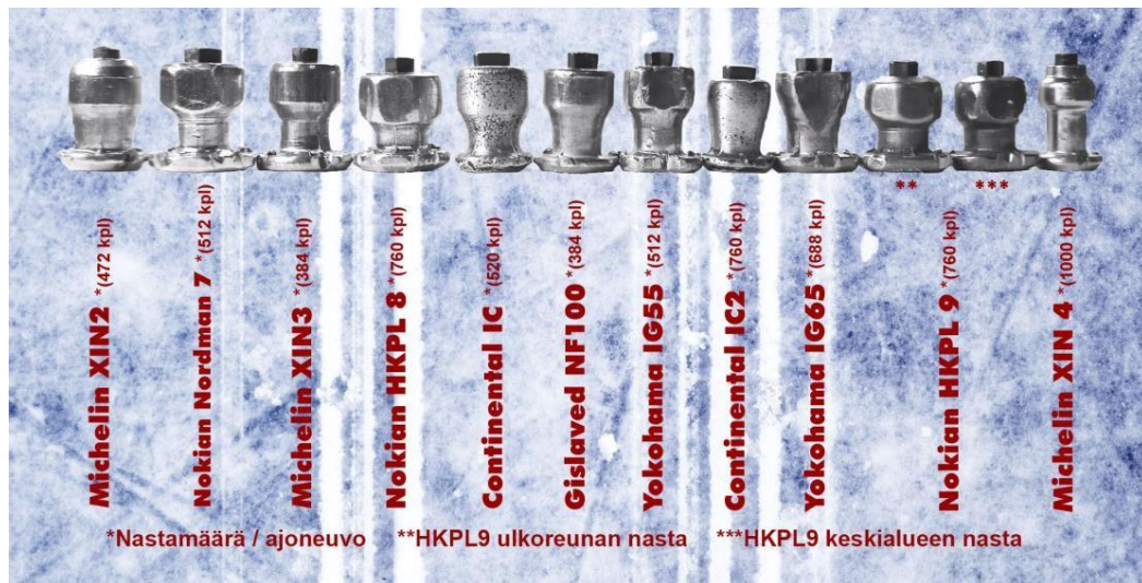
Figure 2. Stud types used in the tyres that were inspected
