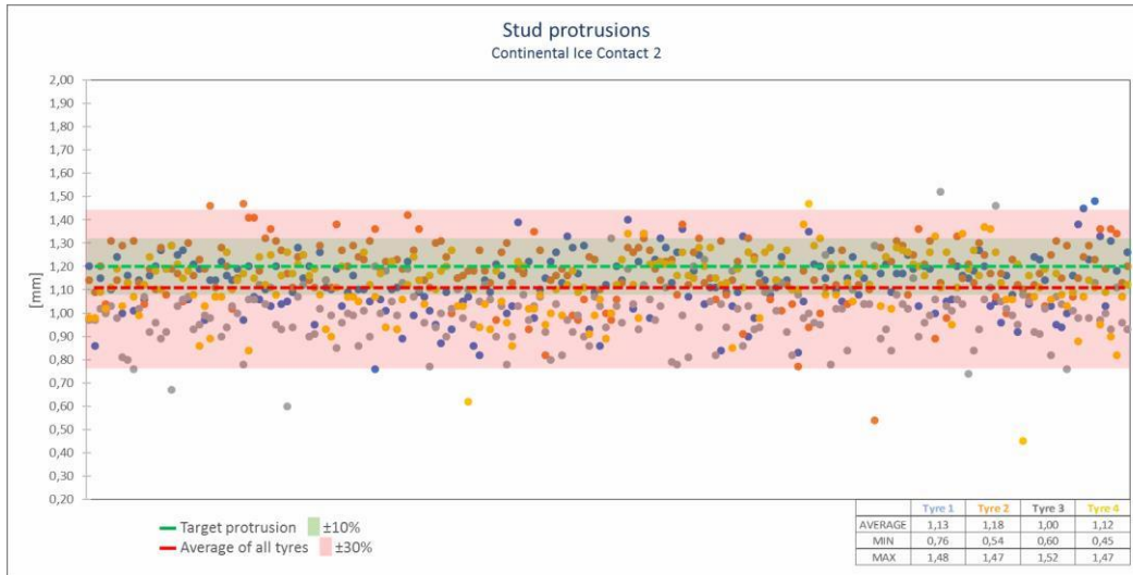
Figure 34. Stud protrusions, Continental Ice Contact 2
