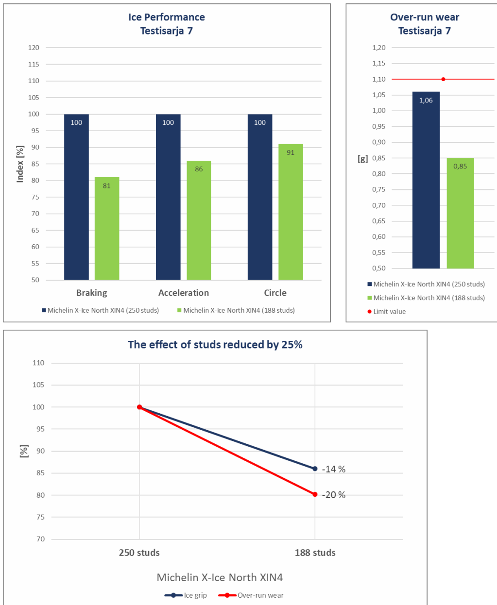
Figure 19. Number of studs reduced by 25%, Michelin X-Ice North XIN4
